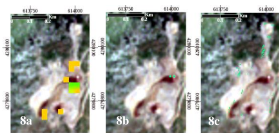
Figure 8. SAM-USGS kaolinite classification maps (a) EnMap (2024/06/19); (b) Sentinel-2 (2024/06/26); and (c) WV3-SWIR (2024/01/06). From left to right, the results were displayed for EnMap, Sentinel-2, and WV3-SWIR when the mineral was classified. The background image is the TCI of Sentinel-2 (2024/06/26). Spectral angle values range between 0.00- 0.125 are given with purple to light blue colors, 0.125-0.225 with medium to light green colours, , and 0.225-0.25 with light orange colour.
